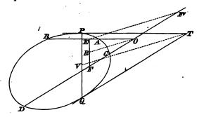
Let TP, TQ be the tangents parallel to OAB and OCD, and such that the angle PTQ is equal to AOC.
